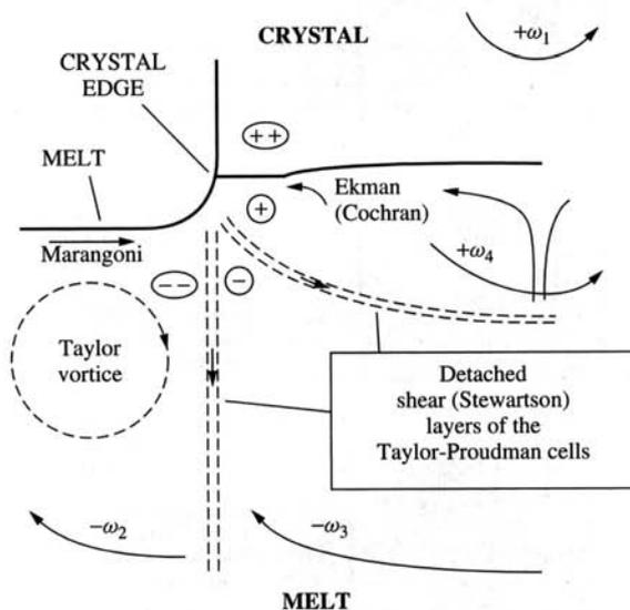
**Figure 4.13** More than six types of flow, differing in direction and/or velocity, below the edge of a Czocharlski-grown crystal for the case of crystal rotation  $+\omega_1$  and crucible counterrotation  $-\omega_2$  above the critical Rossby number (Scheel and Sielawa 1985).
