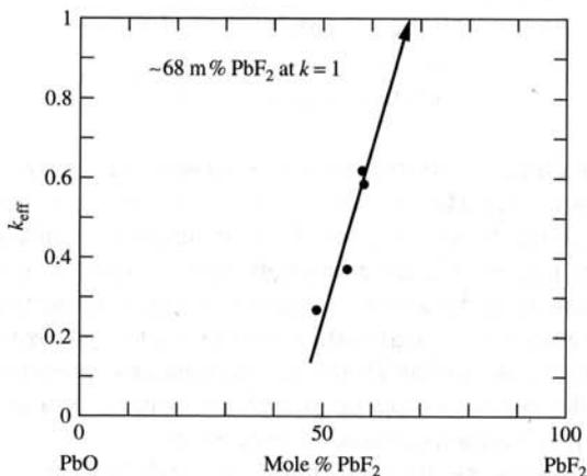
**Figure 4.4** The dependence of the effective distribution coefficient on the PbO–PbF<sub>2</sub> solvent ratio in flux growth of Cr-doped yttrium iron garnet, after Scheel and Swendsen 2001.
