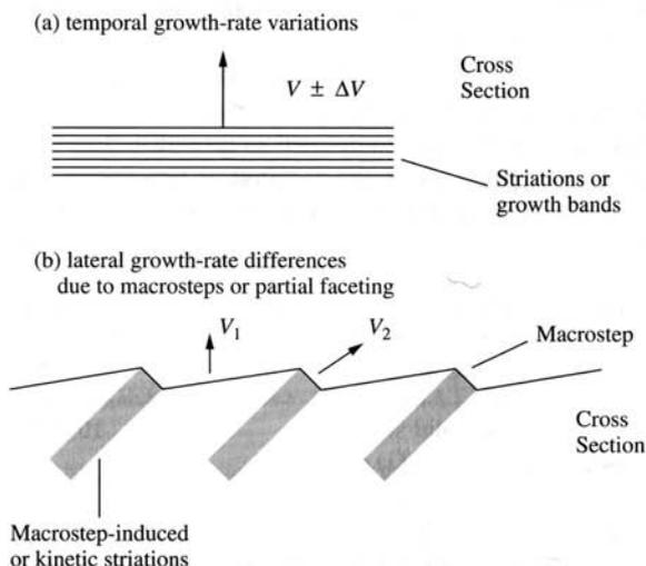
**Figure 4.1** Definition of striations (a) caused by temporal growth-rate and temperature fluctuations as 'thermal striations', (b) caused by macrosteps and lateral growth-rate differences as 'macrostep-induced striations' or as 'kinetic striations'.
