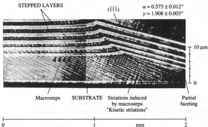
**Figure 4.2** Macrostep-induced striations visible in the etched p-GaAs layers of an 11-layer p-/n-GaAs structure grown by liquid phase epitaxy (Scheel 1980). On the GaAs substrate of  $0.58^\circ$  misorientation first a thick layer is grown, which on the right side shows the transition to the  $\{111\}$  facet, whereas the macrostepped surfaces on the left side cause the striations. Angle-lapped ( $\gamma = 1.9^\circ$ ) and etched, composite differential interference (Nomarski) micrograph.
