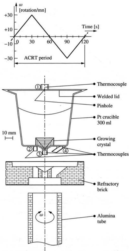
**Figure 4.10** Side view of a 300-cm<sup>3</sup> platinum crucible, with welded lid and slightly cooled spot at crucible bottom for nucleation control, used in the ACRT experiments for growth of KTN crystals (Rytz and Scheel 1982). A typical ACRT period is also shown.
