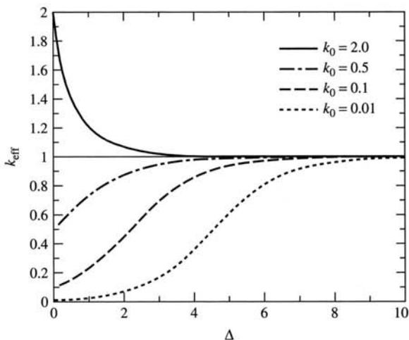
**Figure 4.8** The effective distribution coefficient as a function of the exponent  $(v\delta/D) = \Delta$  from the Burton-Prim-Slichter Equation (4.4) for four values of  $k_0$  (Scheel and Swendsen 2001).
