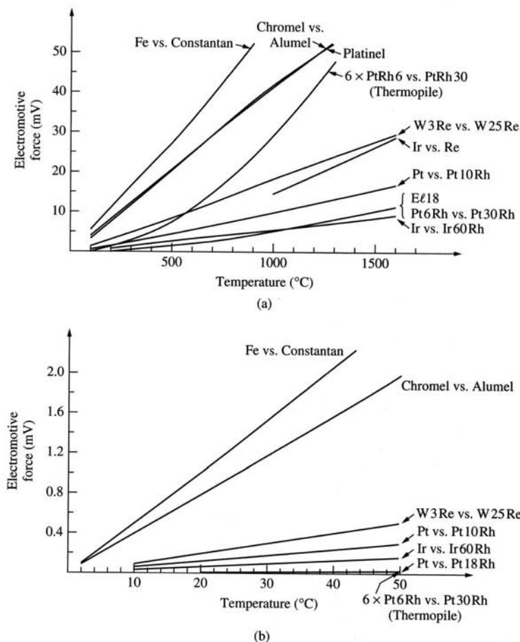
**Figure 4.11** The electromotive forces of various common thermocouples (a) for high temperatures, (b) for the temperature range 0 to 50°C. Note that the thermopile of 6 × PtRh6% versus PtRh30% has a very high sensitivity at high temperatures and practically no sensitivity around room temperature (Scheel and West 1973, from Elwell and Scheel 1975).
