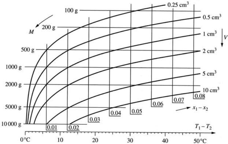
**Figure 4.6** Nomogram to read the experimental parameters for growth of KTN solid solution crystals of a specified maximum inhomogeneity  $x_1 - x_2$  and volume  $V$ .  $M$  = mass of the melt,  $T_1 - T_2$  is the cooling interval (Rytz and Scheel 1982).
