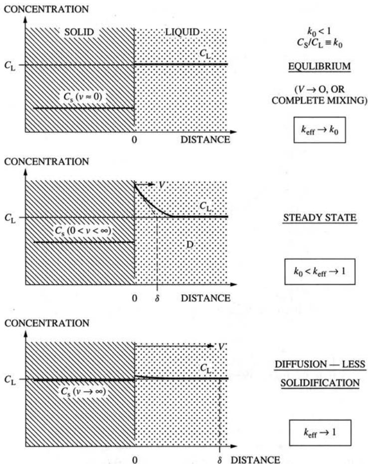
**Figure 4.7** The concentration relations at the growth interface and the effective distribution coefficients for three growth situations: near equilibrium  $k_{\text{eff}}$  approaches  $k_0$ , in very fast solidification  $k_{\text{eff}}$  approaches unity, and in typical crystal growth  $k_{\text{eff}}$  is between  $k_0$  and 1. The diffusion boundary layer thickness  $\delta$  depends on the growth rate  $v$  and on the flow rate of melt or solution.
