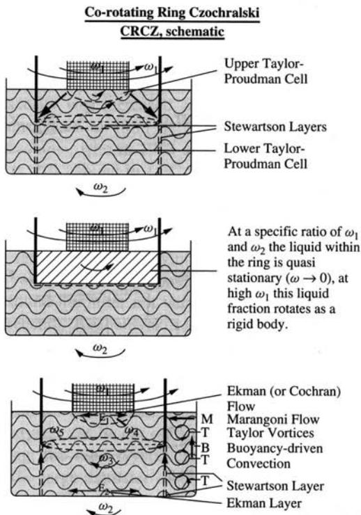
**Figure 4.14** Schematic presentation of the Co-rotating ring Czochralski CRCZ concept where the complex flow region of Figure 4.13 is transferred deeper into the melt and where the liquid fraction within the ring can be separated from bulk melt flow under optimized conditions (Scheel 1995).
