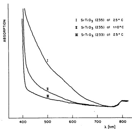
FIGURE 2 Optical absorption of a photochromic brown crystal No. 235 (I), of the same crystal bleached at 110°C (II), and of a nearly colourless crystal No. 233 (III) [ $d = 10$  mm].
