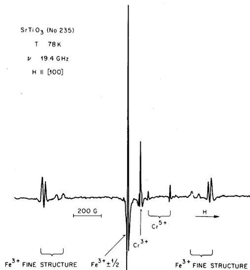
FIGURE 3 EPR spectrum (at 78 K) of the photochromic crystal No. 235.
