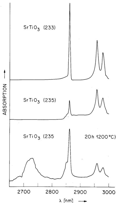
FIGURE 4 Infrared absorption of SrTiO<sub>3</sub> No. 233, of the photochromic SrTiO<sub>3</sub> No. 235, and of the same crystal after annealing at 1200°C [*d* = 10 mm].
