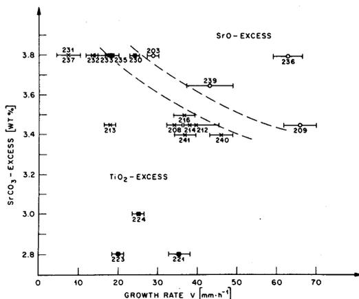
FIGURE 1 Results of X-ray analyses of overflowed melts from experiments with various growth rates and various  $\text{SrCO}_3$  excess in the  $\text{SrTiO}_3$  powder. Large  $\text{SrTiO}_3$  crystals can be grown in the narrow range between the region with  $\text{SrO}$  excess (o) and the region with  $\text{TiO}_2$  excess (x).
