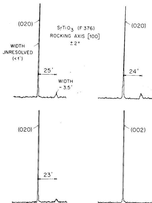
FIGURE 5  $\gamma$ -ray rocking curves of a SrTiO<sub>3</sub> crystal grown from Sr-Li-borate flux.
